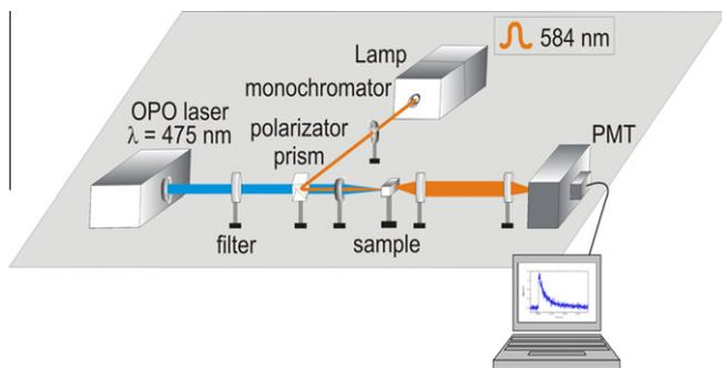
Fig. 1. Experimental setup used in the pump and probe experiments.
