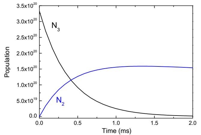
Fig. 5. Simulation of the temporal evolutions of the populations of the  ${}^4\text{F}_{9/2}$  ( $N_3$ ) and  ${}^6\text{H}_{13/2}$  ( $N_2$ ) levels.
